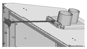
Proceed turning the slide plate tool clockwise to prevent the tool from losing its grip. Push to disengage the slide plate from the top of insert.
