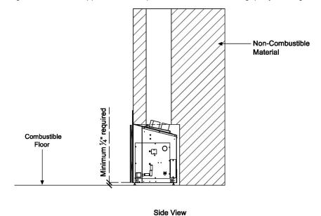
**Raised Platform Option:** To raise the fireplace higher, build a platform for the fireplace to stand on. Platform must be stable and able to bear the full weight of the fireplace. Platform must be constructed out of concrete, metal, or any other non-combustible materials unless you are raising the leveling legs a minimum of ½".
