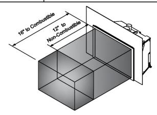
IMPORTANT NOTE: When placing material near the glass, take care to consider fireplace serviceability. It is strongly recommended that any items/materials placed in front of the front (long) glass be movable for easy access to the fireplace during servicing.
