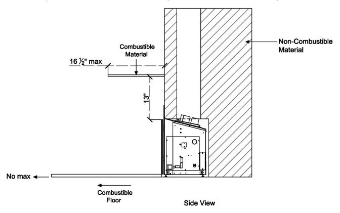
For combustible mantel depth greater than 16 ½", a non-combustible floor or hearth must extend 10" from the unit. Non-Combustible flooring or hearth must remain below the bottom of the surround. A mantel is required to be a minimum of 13" from the top of the front frame.
