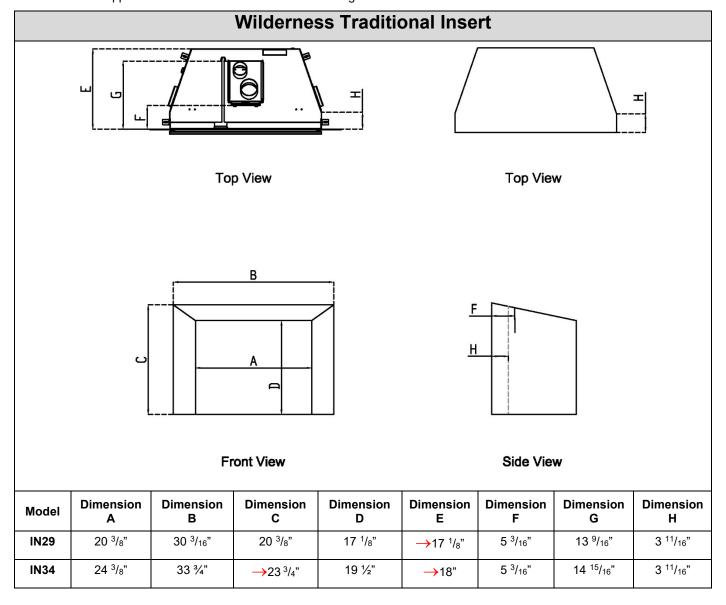
Note: 1/4" Clearance is required on both sides, top, and back of the appliance. These clearances are already calculated into the dimensions shown above.
