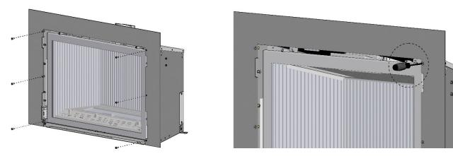
To reinstall the surround, align the six bolt holes on the surround with the six threaded rivnuts on the insert. Start threading each bolt before tightening them all for easier installation.
