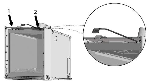
Pull out and then lift to release the keyhole latches. These keyholes are spring loaded and will retract into place once released.
