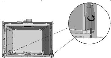
Both left and right sides of the insert have panels located towards the back. Remove 2 bolts for each side panel to remove
