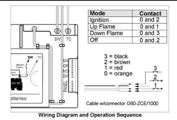
**Mode of Operation:** The external source provides ON and OFF operation only. The Timer/Thermostat handset provides all other functions.
