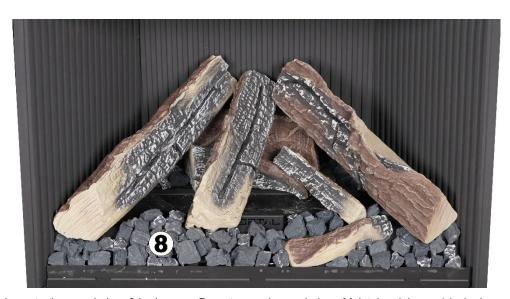
Add the charcoal pieces to the remainder of the burner. Do not cover burner holes. Maintain minimum 1-inch clearance around the pilot behind pilot hood.
