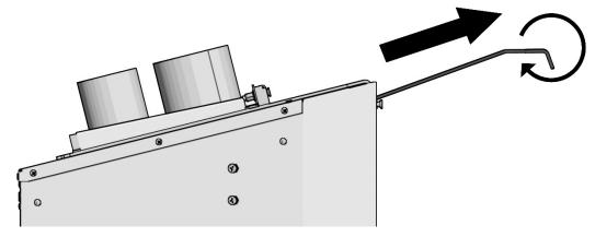
Tilt the glass assembly forward, and then lift up and out.
