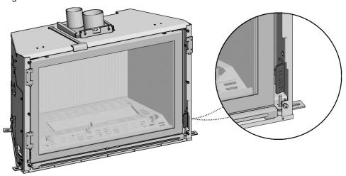
With one hand supporting the glass assembly, locate the two keyholes located at the top of the firebox. Engage the end of the glass tool with the keyholes one at a time.
