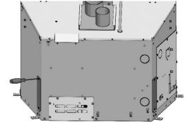
Using the 3mm Allen Wrench, turn the back two leveling bolts counterclockwise to the desired height.
