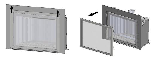
To reinstall the front frame, align the four brackets (two on each side) of the frame with the two top and two bottom bolts, lift up slightly and push decorative front toward fireplace until brackets and bolts are engaged. When properly installed there should be  $\frac{1}{2}$ " gap between the front frame and surround.
