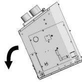
Using a Phillips head screwdriver, turn the 4 leveling bolts counterclockwise to the desired height.
