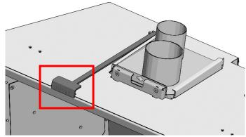
Using a Phillips head screwdriver, remove the two bolts attaching the slide plate. Place the end of the slide plate tool into the cut out on the slide plate.
