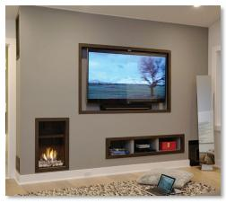
• **Heat Release on a Short Chase**: On most models, the chase above the fireplace can be built as short as 12 inches above the fireplace viewing area. In this instance, there are two ways to approach the heat release; it can be at the front edge or on the top of the chase.
