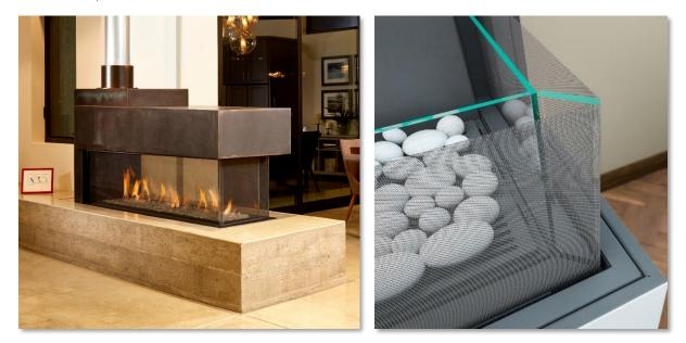
This patented technology incorporates a glass bracket set at a 45° angle at the glass-to-glass connection points. The screen is then wrapped around the viewing area, supported by the glass brackets, and attaches inside the firebox frame at the sides, allowing the fireplace to maintain a completely frameless design.
