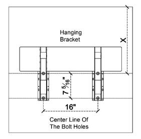
UIAGRAM NOTE: The hanging bracket is shown in the diagram above as a reference point only. The fireplace will not be mounted to the wall until step 3.
