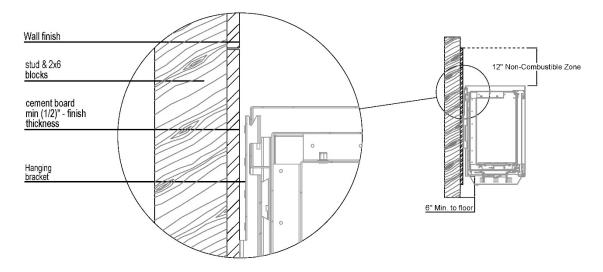
UIAGRAM NOTE: The fireplace is shown in the diagram above as a reference point only. The fireplace will not be mounted to the wall until step 5.
