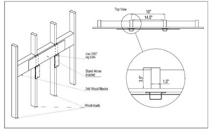
UIAGRAM NOTE: The hanging bracket is shown in the diagram above as a reference point only. The hanging will not be mounted to the wall until step 3.
