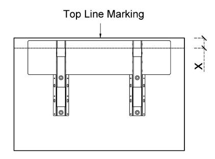
Mount the Hanging Bracket: Center the hanging bracket along the line marking made in Step 2. Using the information in the table below, mount the bracket to the wall using the four <sup>3</sup>/<sub>8</sub>"-diameter expansion bolts following the bolt manufacturer's requirements (bolts are not provided). Recommended bolt length is minimum 3" but may need to be longer depending on project design needs.
