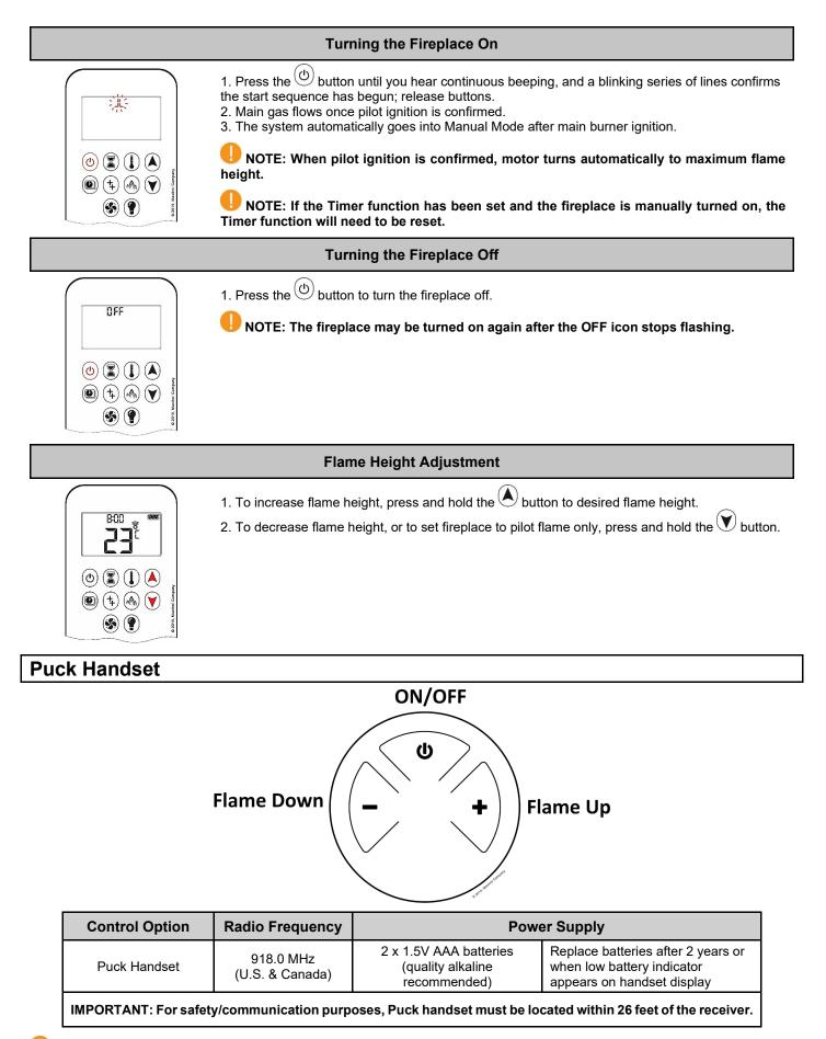
NOTE: Any device that functions using the same radio frequency as the handset will be affected when handset is in use.
