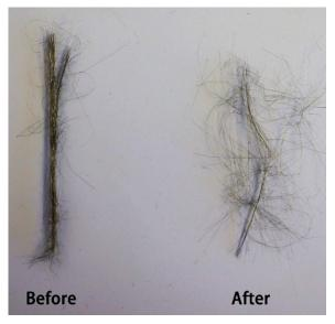
2. Place nickel hair strands on top of the burner holes. Keep nickel strands a minimum of 1 inch from the pilot.
