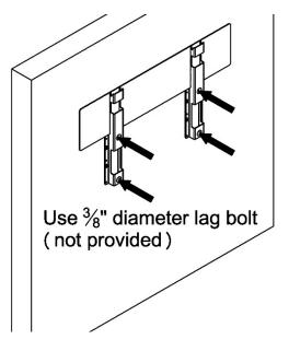
UNOTE: To ensure the fireplace can be installed tightly to the wall, make sure the bolt doesn't stick out more than <sup>5</sup>/<sub>8</sub>" from the wall.
