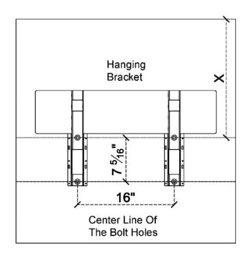
Mount the Hanging Bracket: Center the hanging bracket along the line marking you just made. Using the information in the table below, mount the bracket to the wall using the four <sup>3</sup>/<sub>8</sub>"-diameter lag bolts following the bolt manufacturer's requirements (bolts are not provided). Recommended bolt length is minimum 3" but may need to be longer depending on project design needs.
