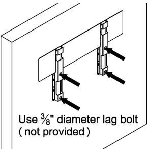
UNOTE: To ensure the fireplace can be installed tightly to the wall, make sure the bolt doesn't stick out more than <sup>5</sup>/<sub>8</sub>" from the wall.
