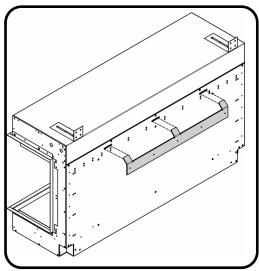
Screw the two top mounted brackets to the wall.
