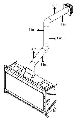
NOTE: The vent clearance diagram above is for illustration purposes only. The Enervex Power Vent is not shown in the diagram and is required for optimal operation of the fireplace.
