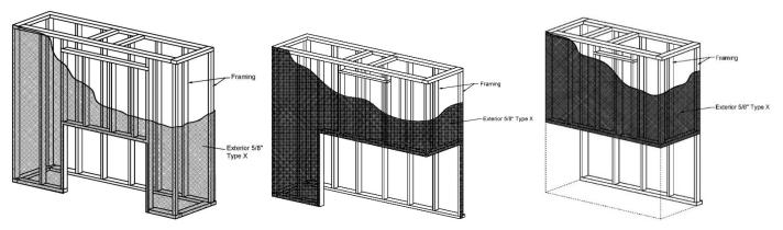
UNOTE: 5/8" Type X Drywall (or equivalent) is not required on the exterior portion of an insulated outside-facing wall.
