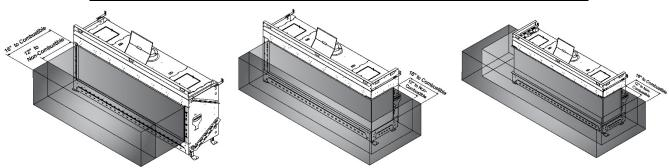
Materials (including combustible flooring and combustible finish material) are permitted below and around the viewing area clearance zone.
