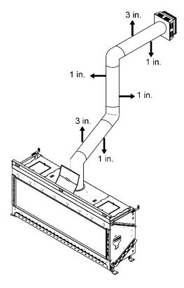
NOTE: The vent clearance diagram above is for illustration purposes only. The Enervex Power Vent is not shown in the diagram and is required for optimal operation of the fireplace.
