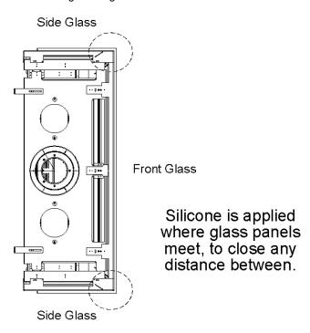
Glass Seal Assembly Diagram
