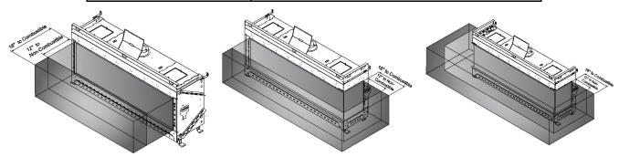
Materials (including combustible flooring and combustible finish material) are permitted below and around the viewing area clearance zone.
