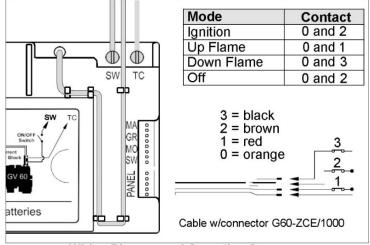
Wiring Diagram and Operation Sequence
