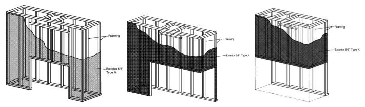
NOTE: ⁵/8" Type X Drywall (or equivalent) is not required on the exterior portion of an insulated outside-facing wall.
