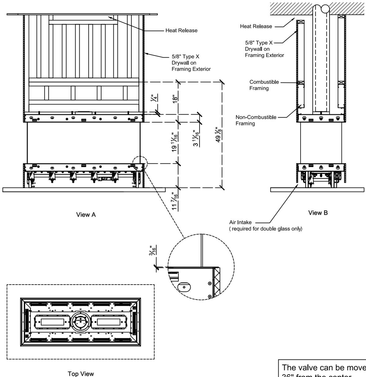
The valve can be moved 36" from the center of the fireplace in any direction
