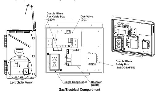
A gas shut-off valve and a 12" gas flex connector are provided with every fireplace. The location of the gas shut-off valve is dependent on local codes and requirements. Check with your authority having jurisdiction for more information.
