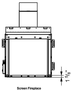
The screen fireplace does not come with legs and can sit directly on the chase floor/platform.
