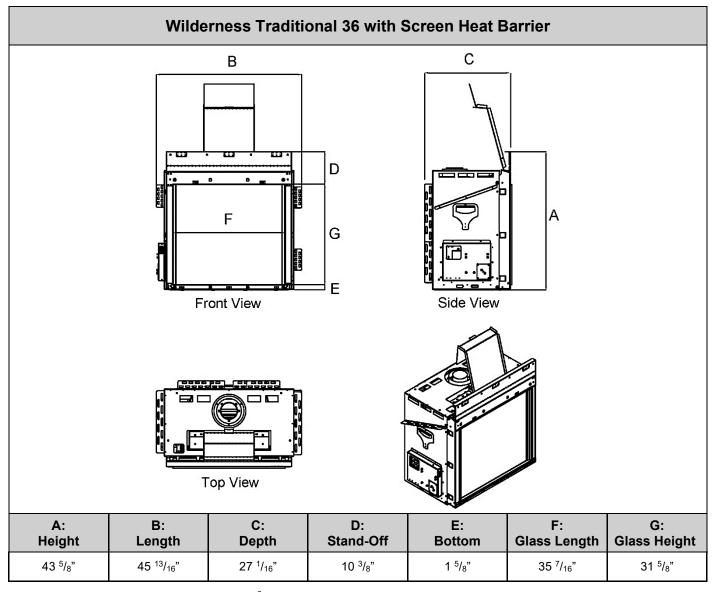
No material is permitted to extend past the  $\frac{5}{8}$ " metal drywall lip surrounding the fireplace viewing area. This area must be unobstructed to allow the heat barrier and inside glass panel to be removable.
