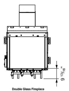
The double glass fireplace has legs to allow for space and airflow for the double glass fans. The legs cannot be cut, removed, or altered in any way. The legs can sit directly on the chase floor/platform.
