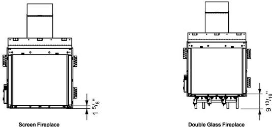
**Raised Platform Option:** To raise the fireplace higher than  $1^{5}/8$ " for screen or  $9^{13}/16$ " for double glass, build a platform for the fireplace to stand on. Platform must be stable and able to bear the full weight of the fireplace. A platform can be constructed out of wood, concrete, metal, or any other solid materials. Platform material is not required to be non-combustible.
