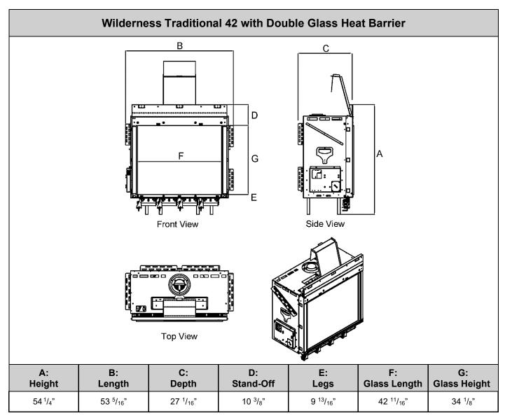
No material is permitted to extend past the  ${}^{5}/{}_{8}$ " deep metal drywall lip surrounding the fireplace viewing area. This area must be unobstructed to allow the heat barrier and inside glass panel to be removable.
